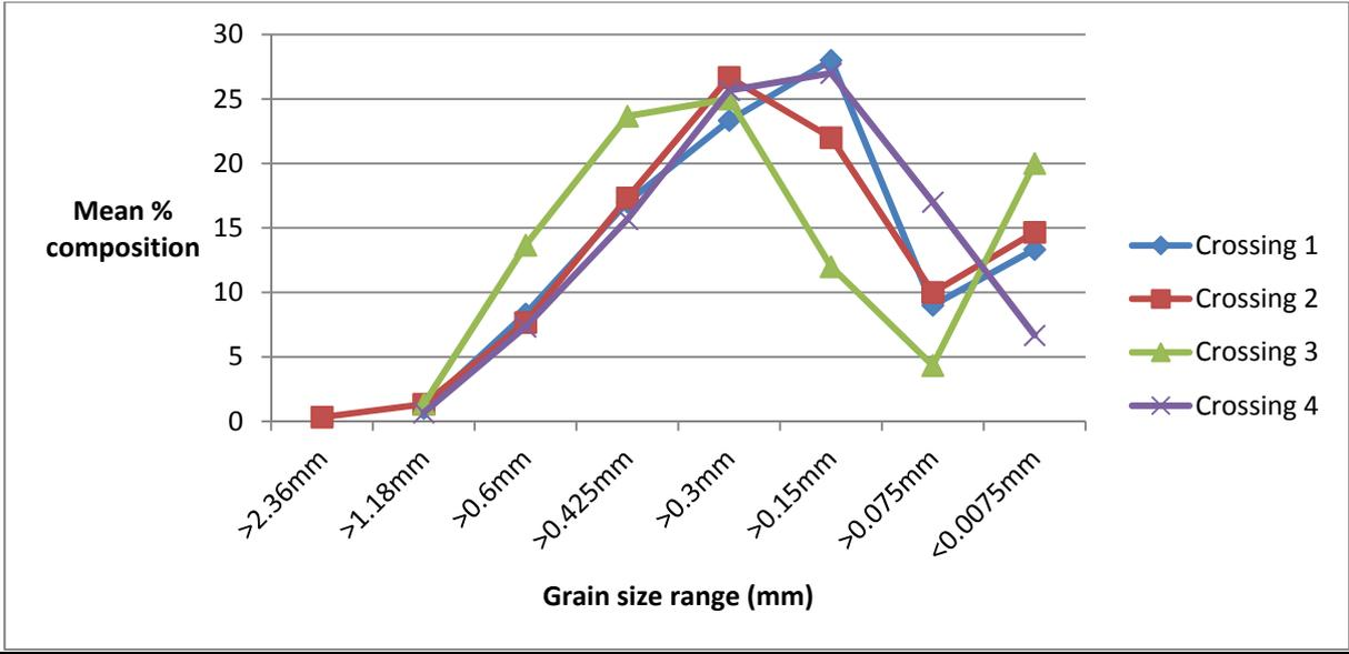
Figure 2 – Mean grain size distribution for creek crossings
